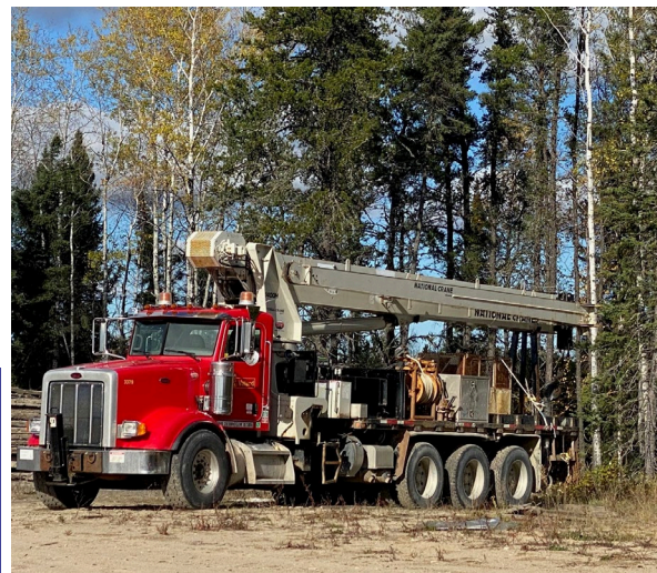
A crane truck, like the one seen here in October, is a versatile construction tool that can lift and move heavy materials around site. It is one of the most recognizable trucks on a construction site, because of its “telescopic boom”.
