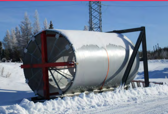
A reactor on its side is waiting to be installed.
