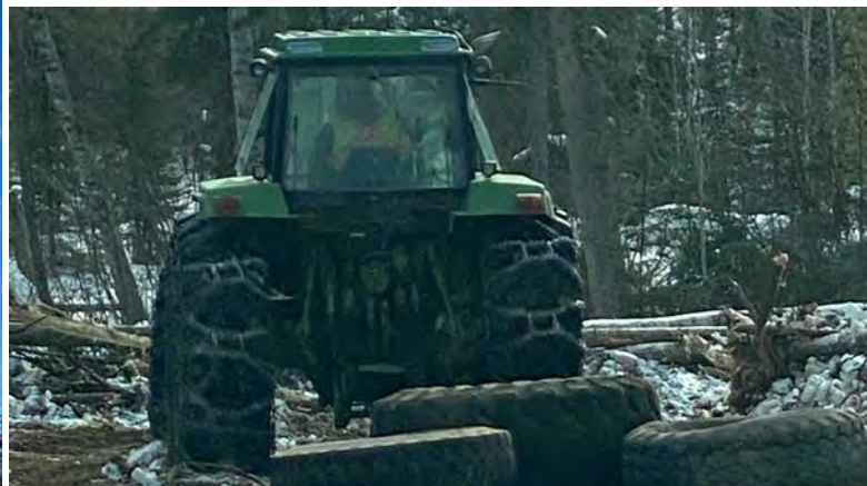
A tractor is dragging tires along an access trail to drive frost deeper into the ground in March 2023. Increasing traffic along relatively bare ground increases the rate of frost penetrating the subsoil. A deep layer of frozen soil improves the access along the ROW and access trails.
