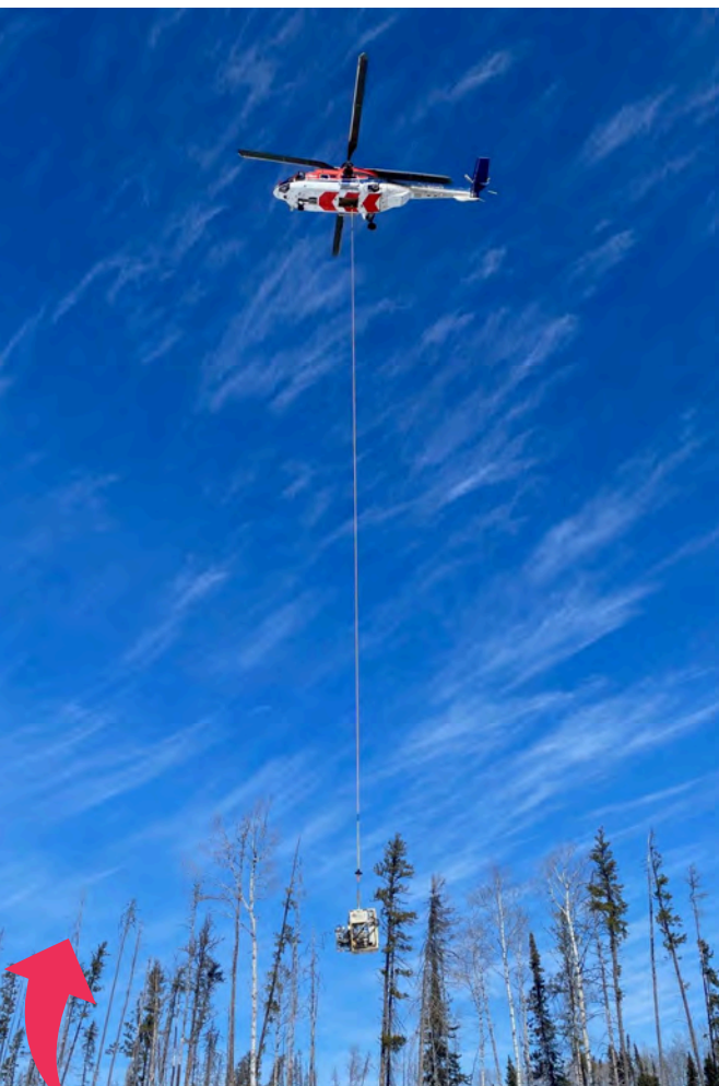
In March 2023, a helicopter longlines gear between Knox camp and Sandy Lake First Nation. "Longlining" is transporting material or equipment via helicopter using a long cable.
