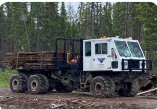
A truck for transporting access mats works between Lac Seul First Nation and Slate Falls Nation. The access mats bridge over soft and wet terrain on the right of way. The use of access mats also minimizes impacts to the land from rutting. The vehicle pictured here is part of a First Nation joint venture business.
